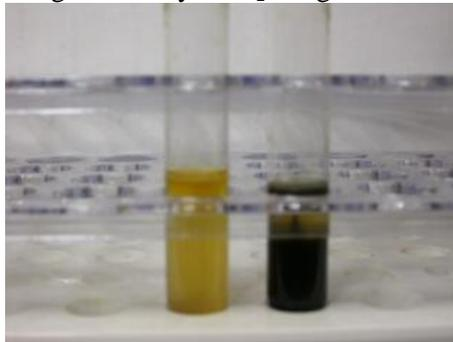
**Figure 5:Hydrogen Sulphide test**
